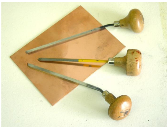
4. Selection of burins and a copper plate for engraving. Wikimedia commons.
